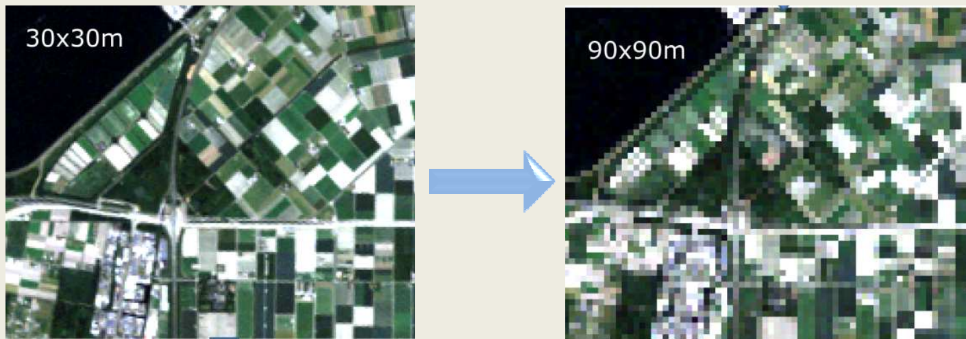
True-colour Landsat-5 TM image of Flevoland (the Netherlands) 26 June 2010, original 30m resolution, and aggregated to 90m resolution.
